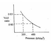
The e-p curve for a soil is shown in the above figure. The coefficient of compressibility (in m<sup>2</sup>/kN) of the soil is
