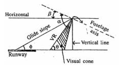
In the above figure shown, "cockpit cutoff angle" is the angle labelled
