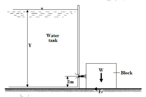
The water jet strikes the block at the vena contracta. The block weighs 750 N, and the coefficient of the friction between block and floor is 0.24. The orifice's coefficient of discharge (C) is 0.60, and its coefficient of contraction (Cc) is 0.62. The minimum height to which water must rise in the tank (y in Fig.) in order to start the block moving to the right is
