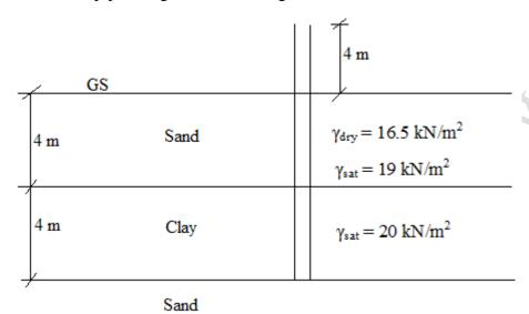
If the dry sand is excavated, then the depth at which the effective stress at the bottom of the clay layer will become zero is
