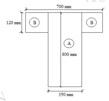
If the section is subjected to a torsion of 150 kNm, assuming the plastic theory, the approximate ratio of the torsion carried by rectangular portions A and B i.e.  $T_A \ / \ T_B$  is
