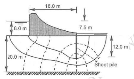
The flow rate in  $m^3$ /day per metre length (upto 2 decimal places) is \_\_\_\_\_\_ ( Take  $k = 5 \times 10^{-5} \text{ m/s})$
